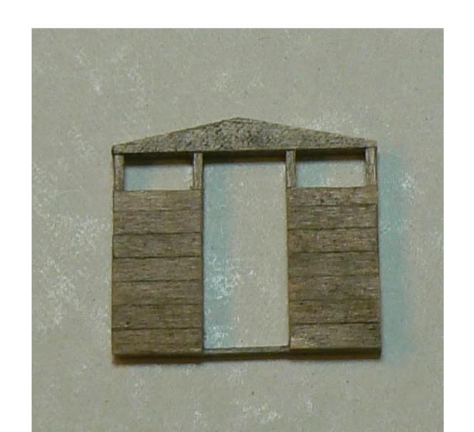
Glue the wall of the cabin together, paint and letter. The lettering here is done with dry transfer lettering.
