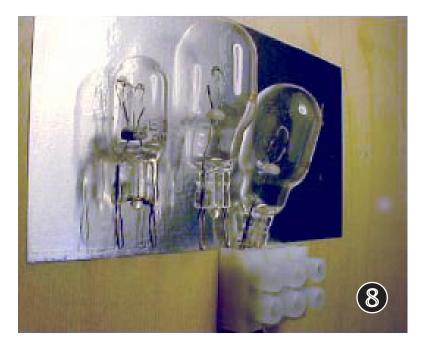
There are other lamps in addition to the 3156 that are wedge base construction and will work for model railroad current limiting applications. There are three physical sizes that could be used, and they are seen in Photo No. 8.
