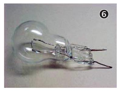
Photo No. 6 is an example of the type of lamp construction to avoid. Note that the leads on this lamp are only about a half inch long, and were reduced in cross-section during the manufacturing process. The leads are also weakened by bending near the glass. The plastic collar has been removed from this lamp.
