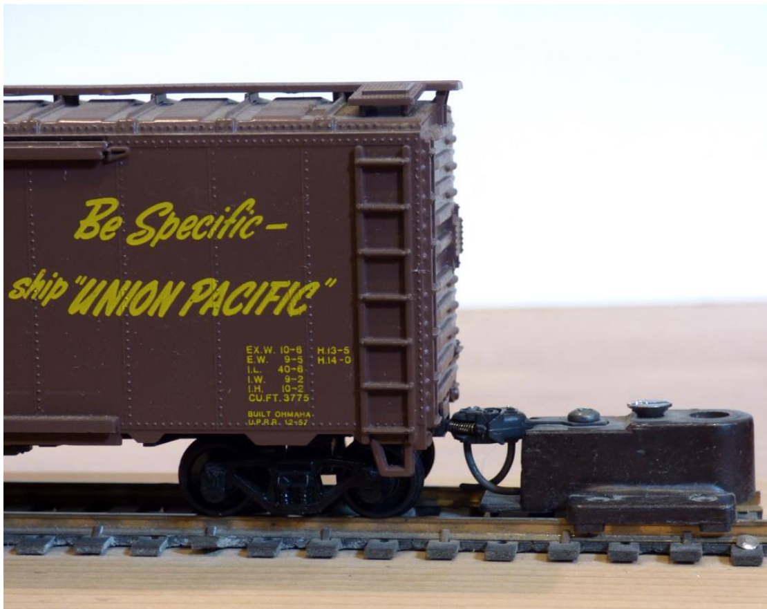
Figure 4: Testing the coupler height on a boxcar using the Kadee gauge.
