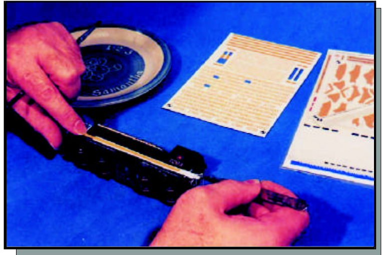
Figure 2: TECHNIQUE USED TO SLIDE DECAL OFF CARRIER FILM AND ONTO THE MODEL
