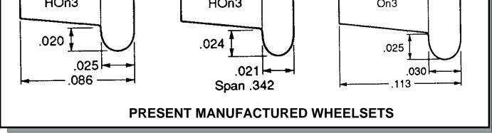
Traditionally, narrow gauge manufacturers have made much finer than standard flanges, only the old Binkley trucks are to exact standard.
